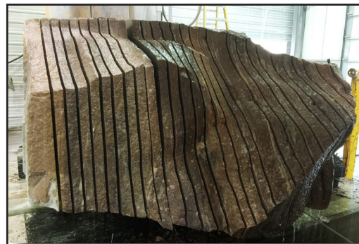
The Sioux Quartzite stone is actively being cut at the quarry in Jasper, MN.
